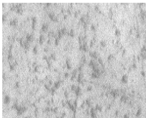
Fig. 4. Optical micrograph of the \text{Ge}_{13}\text{Sb}_5\text{Te}_{82} sample after the thermal treatments up to point B in Fig. 3 (Optical magnification: 1000 \times ).
